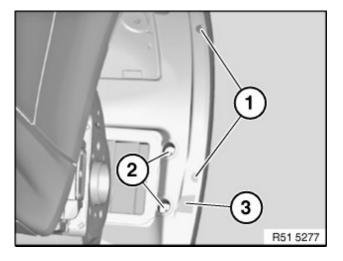
Release screws (1 and 2) and remove right wheel arch cover (3).
