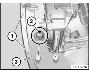
Release screws (1) and plastic nuts (2) on left wheel arch cover (3).
