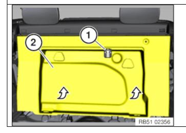
Slide the locking slide for the wind deflector (1) upwards.
