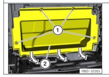
Remove the four plastic rivets (1) from the luggage compartment partition wall. Remove the partition wall.
