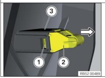
If necessary, replace the defective clip (2) from the backrest side section.
