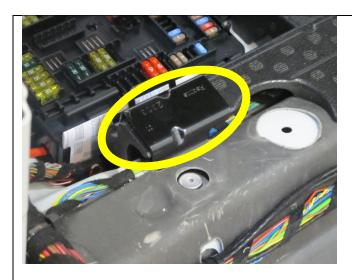
Install P/N 51 47 7 363 430 (bracket for the "thief-proofing flap") using two blind rivets (P/N 07 14 7 265 872).
