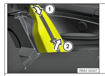
Unfasten the rear safety backrest and tilt it forwards. Pull the safety belt towards the middle and place it over the head restraint.
