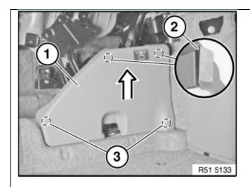
Slide up the trim for the main bearing on both left and right sides of the luggage compartment.
