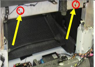
Install both wind deflector stops in the areas highlighted in red, using one self-tapping screw for each side. Note: The stops are left- and right-side specific.
