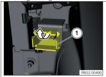
If necessary, replace the defective clip (1) from the body.
