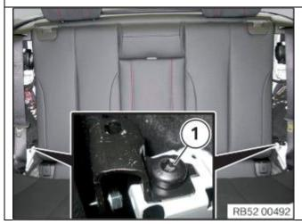
Unlock and tilt the back backrest forward. Remove the screws (1) (the screws must be replaced).
