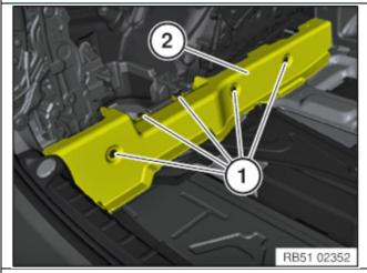
Remove the three plastic rivets (1) that are exposed, facing the center of the luggage compartment.
