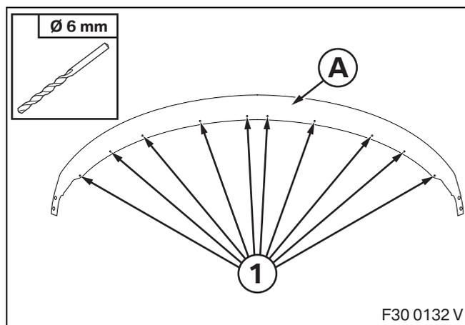
Drill front splitter **A** at the ten pre-illustrated drill hole points (1) using a **6 mm diameter** drill bit.
