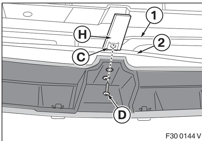
Slide C-clip **C** onto installation plate **H**.
