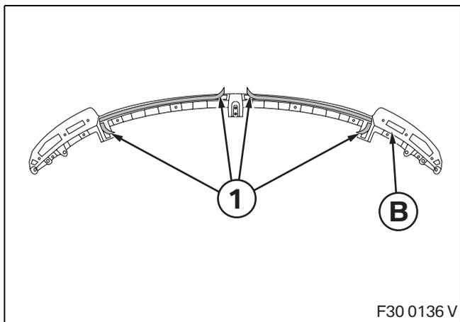
On the back of adapter **B**, fold the protective film (1) on the adhesive strips outwards at the ends.
