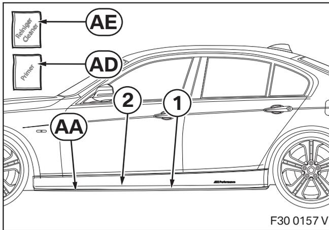
Press left side sill attachment section **AA** upwards and using a suitable tool draw a line (1) at the upper edge of left side sill attachment section **AA** on the side sill.
