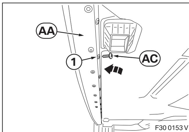
Screw oval-headed screws **AC** into the pre-drilled holes (1) on left side sill attachment section **AA**.
