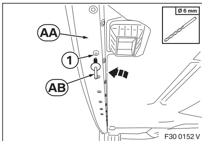
▶ When drilling, note the maximum drilling depth. ◀
