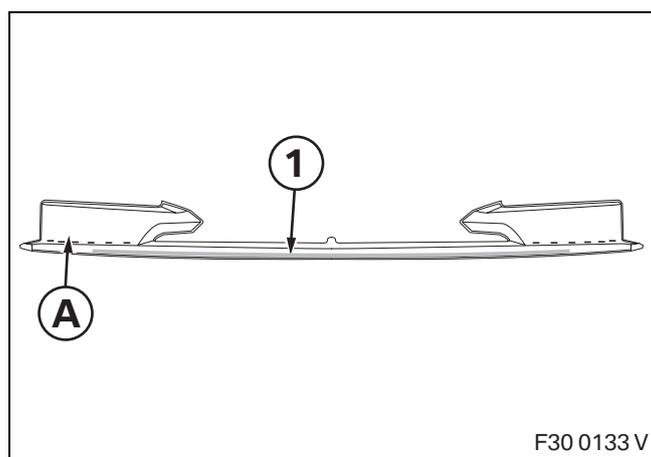
Only prime the bonding surfaces that come into contact with the adhesive strip of adapter **B**. ◀
