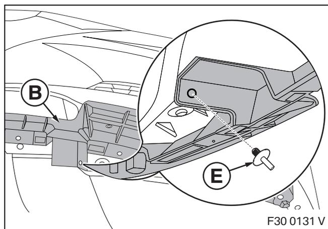
Secure adapter **B** using blind rivet **E**.
