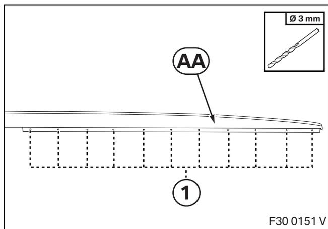
Carefully drill the narrow surface of the side sill at the 11 drill holes (1) on left side sill attachment section **AA** using a **3 mm diameter** drill bit.
