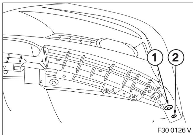
Remove the screw (1) and rivet (2).
