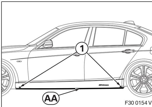
Allow left side sill attachment section **AA** to engage in the rear side sill and align it forwards.
