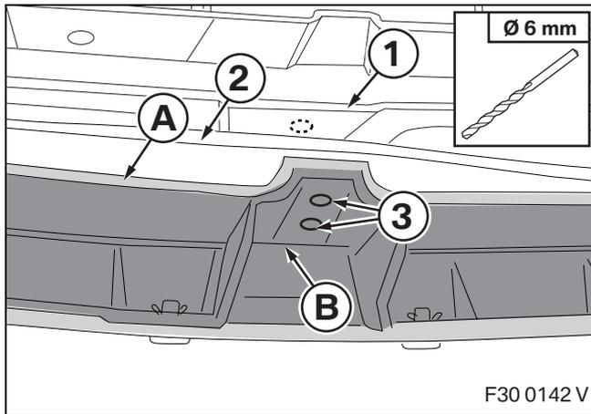
⏏ When drilling, note the maximum drilling depth. The level (1) must also be drilled through. ◀
