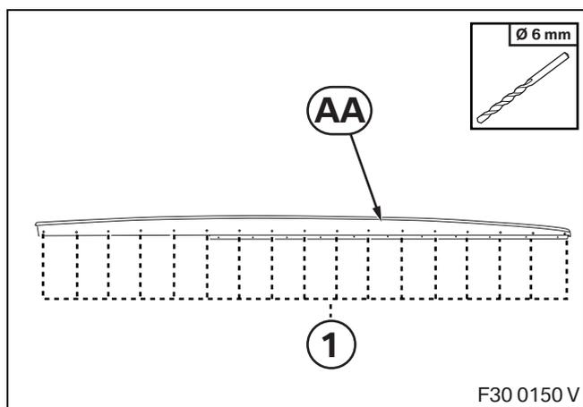
Carefully drill the side sill at the 17 drill holes (1) on left side sill attachment section **AA** using a **6 mm diameter** drill bit.
