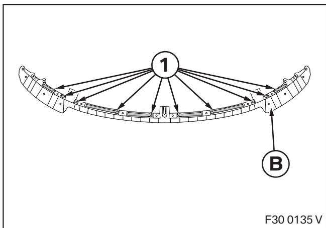
On the front of adapter **B**, fold the protective film (1) on the adhesive strips outwards at the ends.
