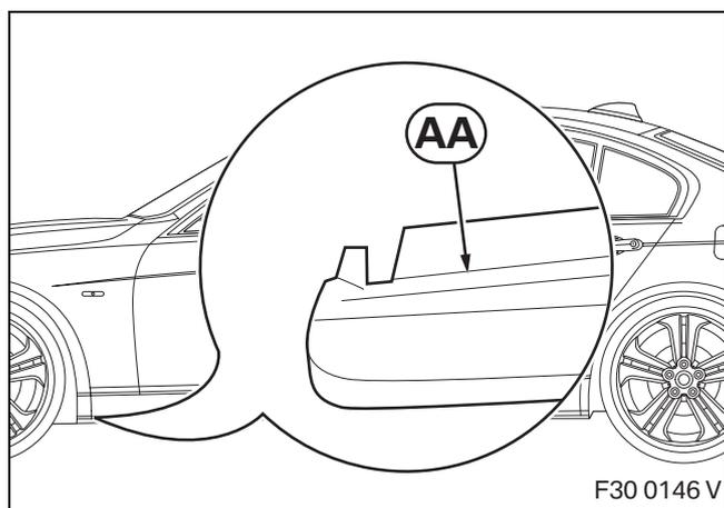
Secure left side sill attachment section **AA** on the front to the side sill.
