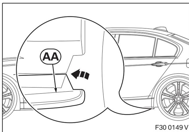
▶ The bonding surfaces must be completely clean, dry and free from grease. ◀
