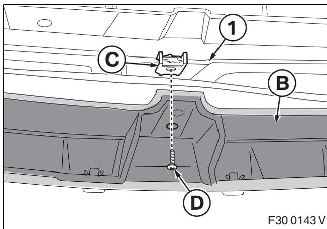
Position C clip **C** on the edge of the level (1). Screw Torx screw **D** through adapter **B** into C-clip **C**.
