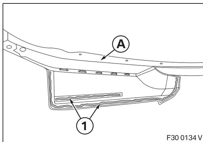
Apply Betalink (1) at the points indicated on the inside of front splitter **A**.
