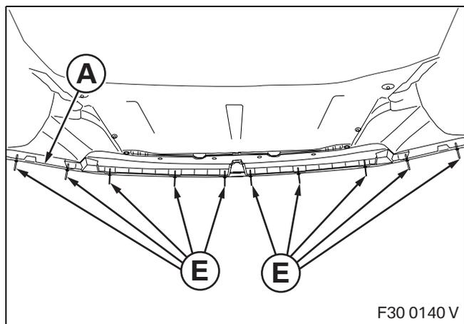
Secure front splitter **A** from underneath using ten blind rivets **E**.
