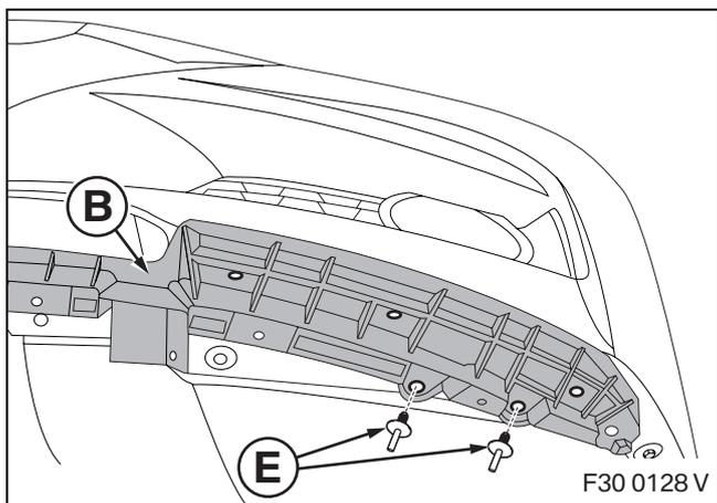
Secure adapter **B** using blind rivets **E**.
