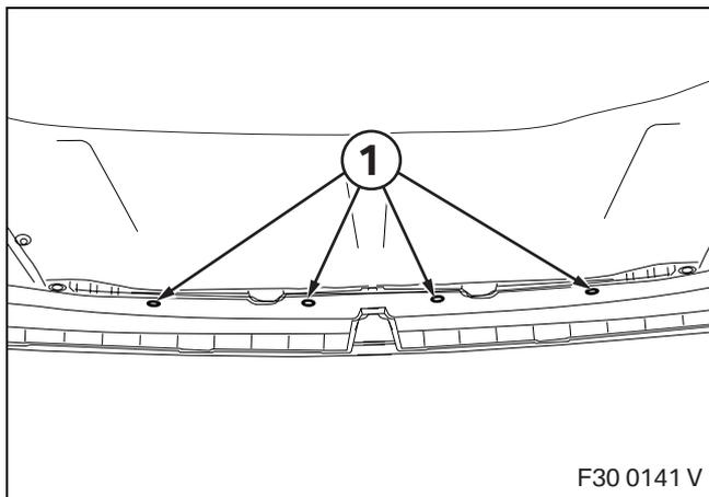
Remove the four expanding rivets (1).
