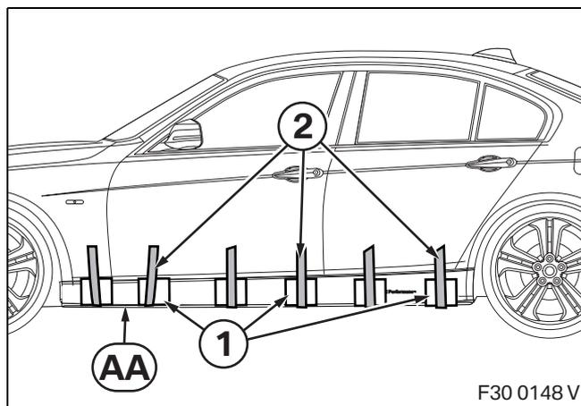
▶ In order to avoid damage caused by adhesive surfaces, the M Performance side sill film must be protected with suitable materials (1). ◀
