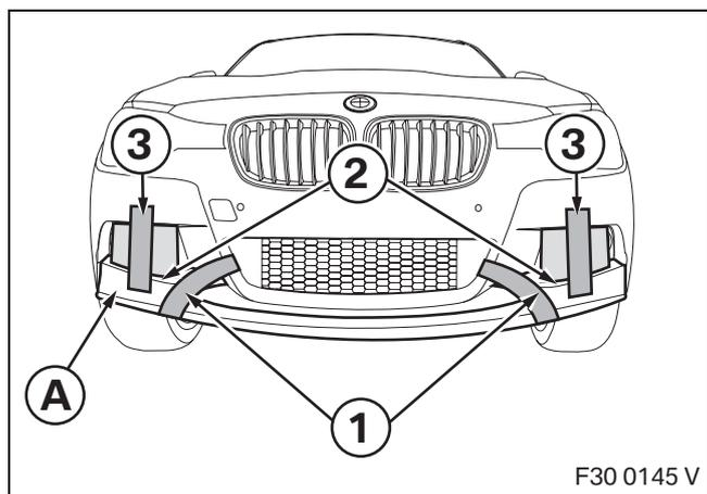
Secure front splitter **A** using suitable adhesive strips (1) to the front apron.
