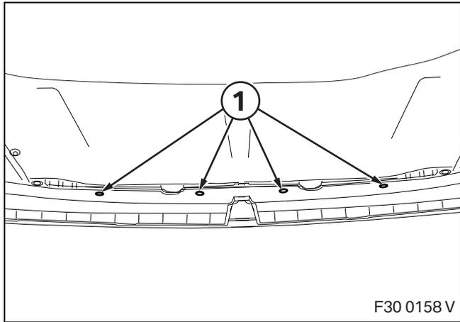
Reinsert the four expanding rivets (1).
