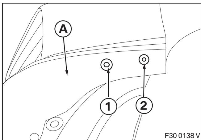
Tighten or insert the existing screw (1) and rivet (2) on the outer side of front splitter **A**.
