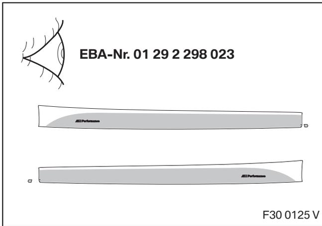
▶ Before installing the M Performance Aerodynamics package side sill, the M Performance side sill films must be installed in accordance with the installation instructions with part number 01 29 2 298 023. ◀
