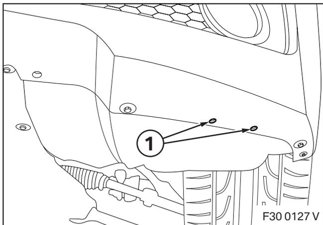
Remove the rivets (1) on the left and right-hand side.
