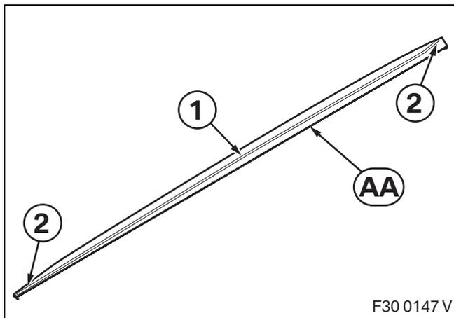
Remove the backing film of the adhesive strip (1) at the ends (2) of left side sill attachment section **AA** and fold outwards at an angle of 90°.
