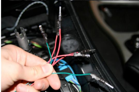
The third and last set of connectors are the power connectors. There are 6 leads total, 3 male and 3 female. Also note that two of these are marked green, and the other four are marked red. Also note that two of the four red connectors bear a black stripe. The green male connector corresponds to the green female connector, the red/black strip connector's male and female connections also coincide and the remaining red connectors also coincide.
