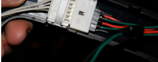
Step 7: Connect the remaining female pin connector to the blue module. Again note the orientation of the connector and wires!
