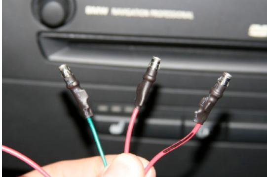
Step 3b: The pins should be lsde in left to right in the following order: green, red, red/black. They should seat snuggly in the molex connector and should not touch. Make sure the red/black wire is furthest to the right. Green is ground.
