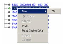
The FDL is displayed as a sub-element of the relevant CAFD entry in font colour orange after the action has been executed.
