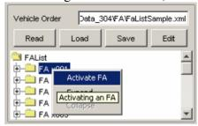
• The vehicle order is set to active and the vehicle profile is calculated and displayed.
